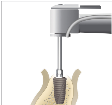
By hand-piece 20rpm / 35N-cm
